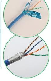
Wrap the drain wire around the jacket of the cable. Make sure the drain wire makes contact with the shielded housing when cover is installed and closed. Use a zip tie to tighten and lock the cover to the housing. Termination is complete.
