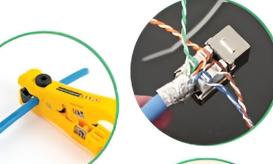
Place conductors into termination slots according to wiring scheme colors and separate pairs using wedge protrusions on connecting block.
