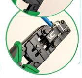
Firmly squeeze the handles together. Release the handles and repeat this step to ensure a proper termination.
