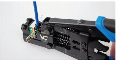
Insert prepared jack & cable assembly into the I-Punch Tool
