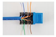
Remove up to 2 inches of the jacket from the cable with a cutter or a stripper. Separate all twisted pairs from each other. Preserve the wire pair twists as close as possible to the point of termination. Determine the wiring scheme and properly align all four cables accordingly on the jack. Keep the cable jacket as close to the connector as possible.
